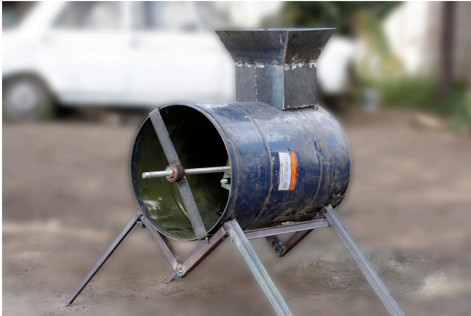
Prototype 2 uses blades similar to the maize grinding machines
