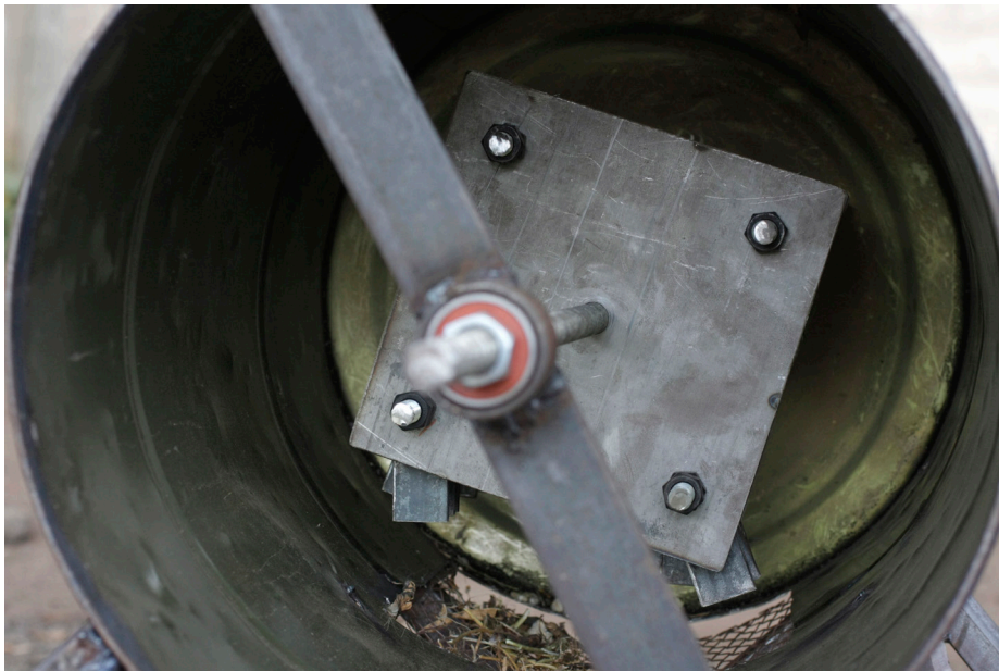
Detail of rotating mechanism inside the drum
