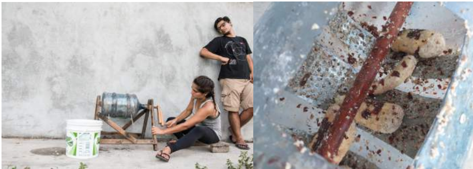
Tumble built using a water cooler jug — Perforated strips with larger teeth were placed circumferentially
