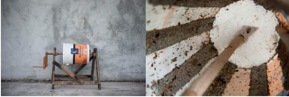
Tumbler built using a water bucket — Perforated strips with smaller teeth were placed axially
