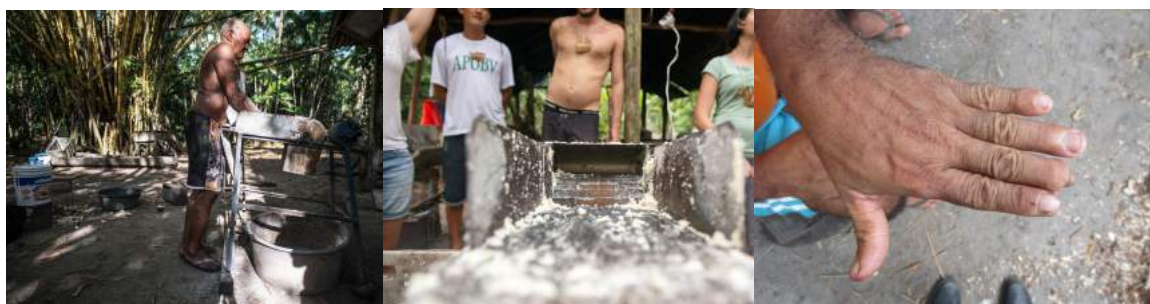
Grating of cassava using an electric grater — No guard is fitted to the grater — Injuries are common but could be addressed with simple modifications
