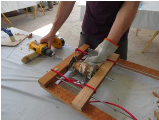
Two sections of studding were mounted parallel within a wooden frame to create a runner on which one section of the check could be mounted and slide. A bungee cord mounted in two places was used to provide a clamping effect between the two chucks.
