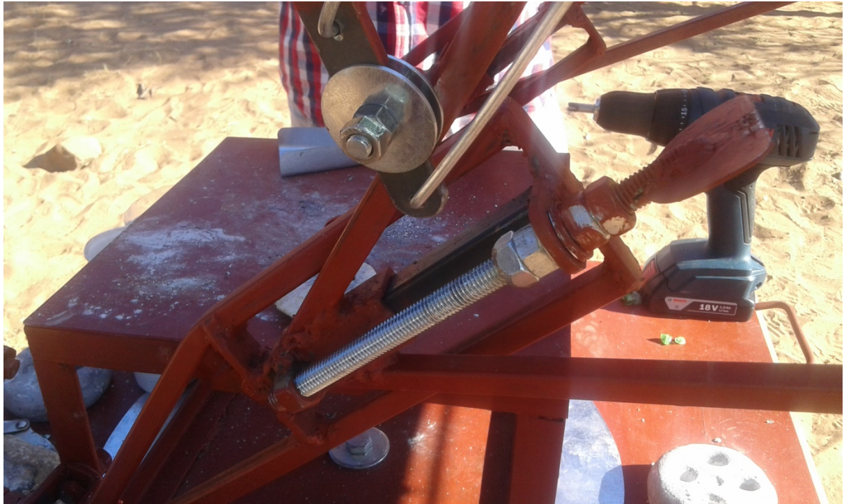
Up and down mechanism using a screw for adjusting the focal distance.
