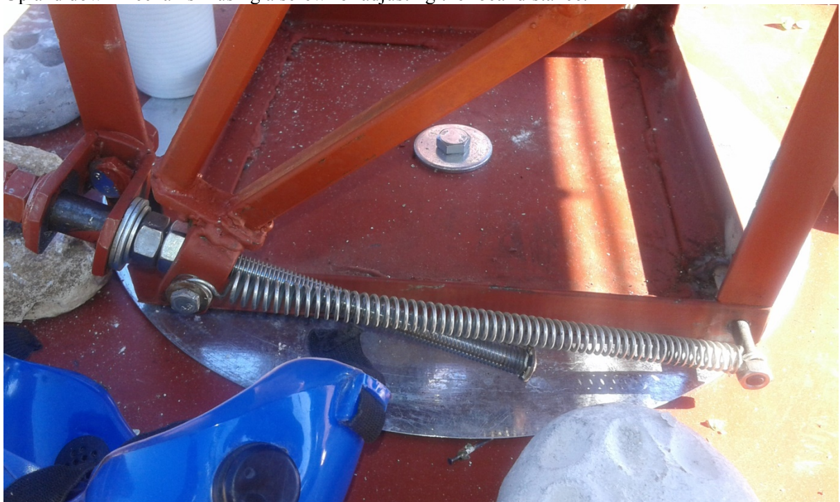
Spring mechanism for adjusting the direction of the lens or for a swing movement.
