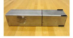
3. Place the metal in the vice. Use the hacksaw to cut along the line drawn such that a 3.5" (9cm) piece of metal tubing is produced.
