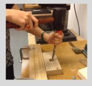
Remove material. Use a smaller chisel (3/4" or 1.8cm in this case) to remove wood inside the hole. Hold the chisel at an angle with the beveled side down. To make cuts in the material, hit the angled chisel with the mallet or wood block. Chisel towards the center of the hole. Remove small pieces of wood at a time to avoid splitting the wood, and cut in all directions.
