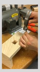
16. Assemble the final press by sliding the ejector piece into the cup so the tubing sticks out the bottom and the sheet metal square is resting on the bottom of the cup. The cup then is placed on top of the wooden table with the ejector going through the hole in the wood.
