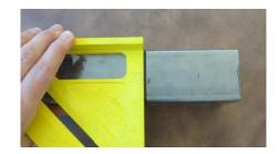
2. Mark the same line along all sides of the metal tubing. Also, mark a ½" (1.3cm) long line starting at the top of the tube and going down along every corner.
