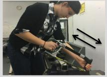
4. Use the hacksaw to cut downward along the ½" (1.3cm) lines drawn at the corners to form the tabs.
