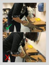
Starting the cut. Place the saw on the cut line. Pull the saw back along the top edge of the wood until a groove is formed. This will help guide the blade as you start sawing.
