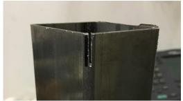
Place the metal piece in a table vice vertically. The larger 4" x 2" x 2" (10cm x 1.3cm x 1.3cm) square metal tubing will have its tabs bent inwards, while the 4" x ½" x ½" (10cm x 1.3cm x 1.3cm) metal tubing will have its tabs bent outwards.
