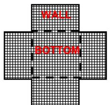
13. Fold up the sides of the baskets to form the walls. Use small pieces of thin wire to tie the walls together.
