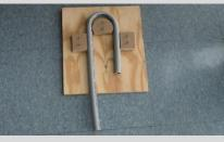
Cut out 3 small circles of fine wire mesh. Wrap these around the long end of three of the siphons and secure with some thin wire. These will act as filters so that the siphons do not fill up with debris.
