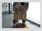
*Letting the PVC cool in the jig.* Keep the piece of PVC in the jig until it is cool to the touch and does not bend easily.
