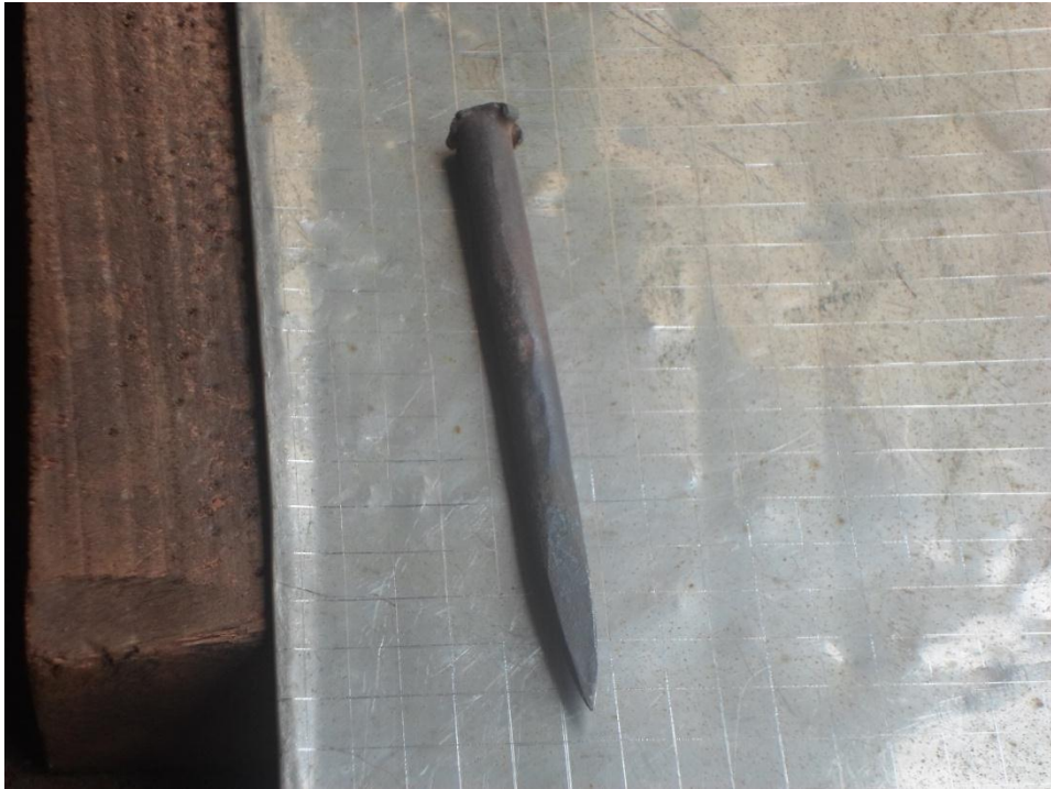
Figure A9: Punch for Making Holes
