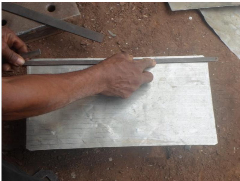
Figure 3.2: Marking out of sheet
