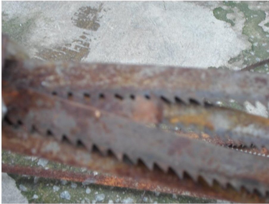
Figure A7: Saw For Making Grating Surfaces DD and EE
