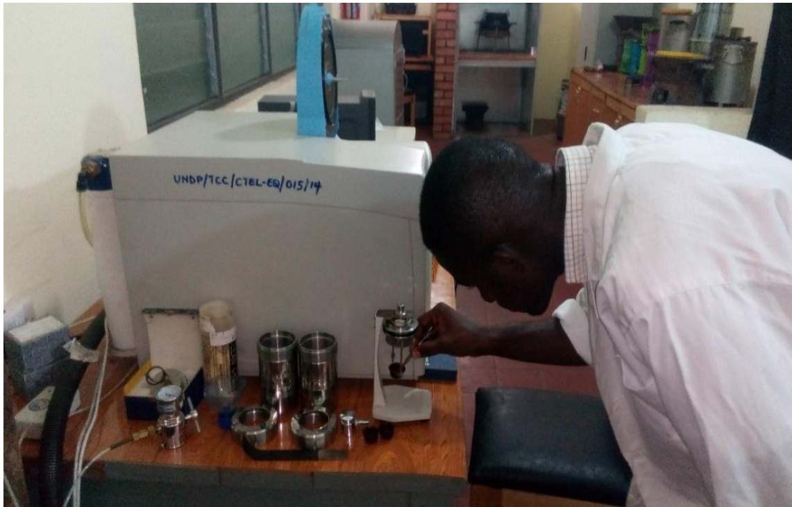
Plate 3.3: Picture showing researcher winding wires over electrodes on the oxygen bomb of the bomb calorimeter.
