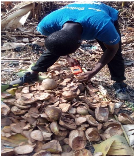
Plate 3.1: Field measurement of moisture content using the wood moisture meter.
