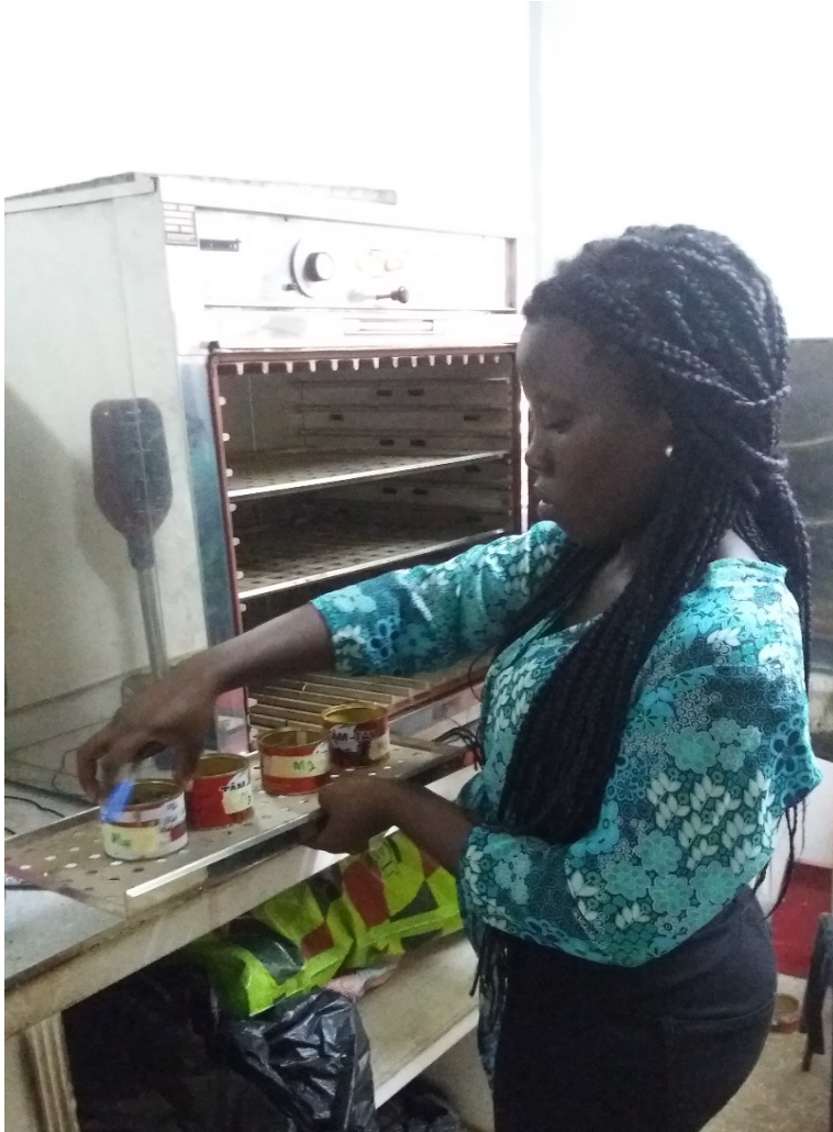
Fig 2: Soil moisture content and bulk density determination
