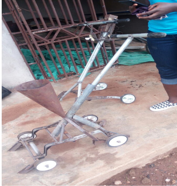
Fig 3.1 Prototype of a two-row groundnut planter, New Longoro
