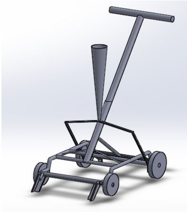
Fig 3.2 Computer aided drawing of the prototype of the two-row groundnut planter.
