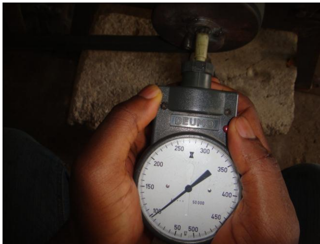
FIGURE 12: Speed reading using a Tachometer
