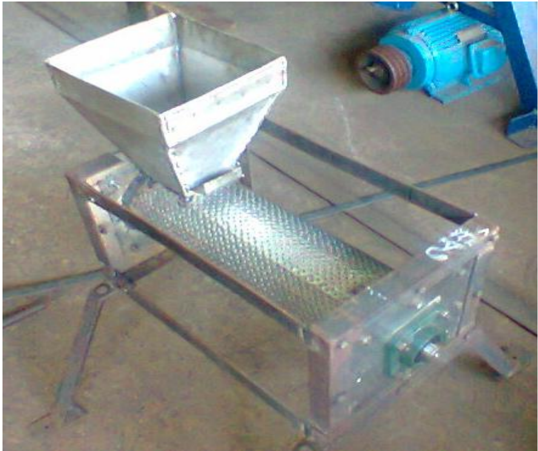
FIGURE 6: Framework of machine at its initial stage of construction
