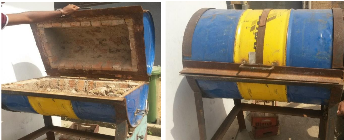
Figure 1. 2 (a) Opened previous furnace design (b) closed old furnace
