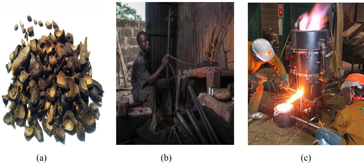
Figure 1.1 (a) Palm kernel shells (b) A local blacksmith using coal (c) Cupola Furnace
