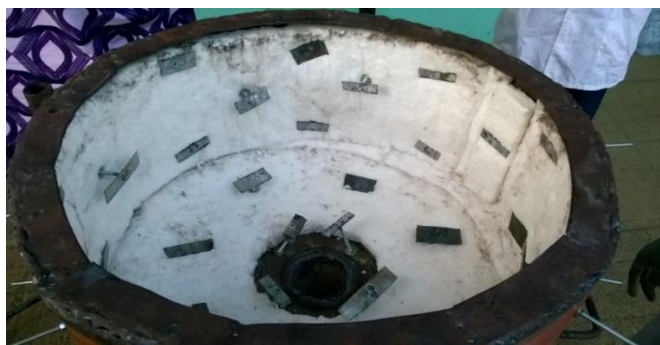
Figure 3. 3 Glass wool held in place by screws.
