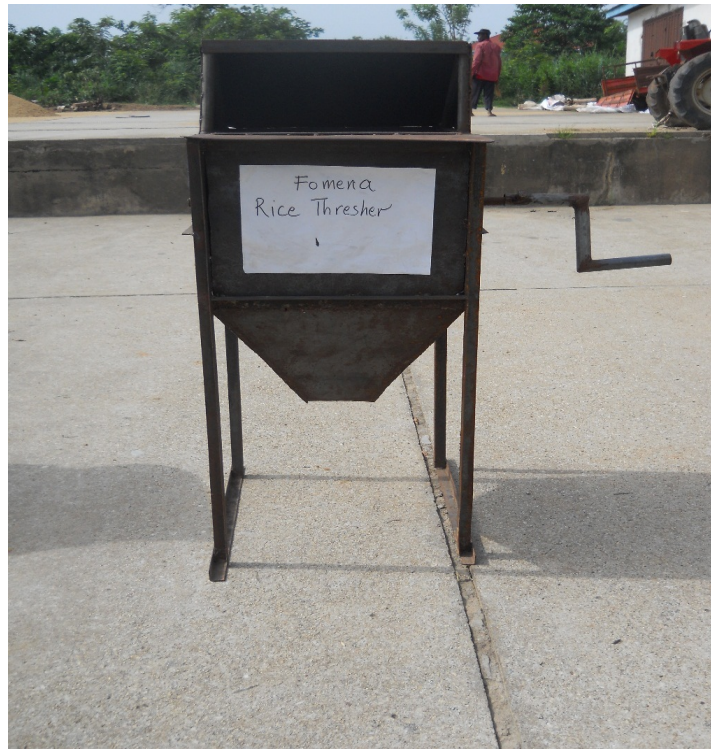
Fig 1. A hand operated rice thresher (Fomena)
