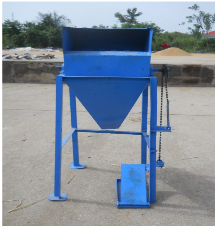
Fig 2. A foot operated rice thresher (Konongo)
