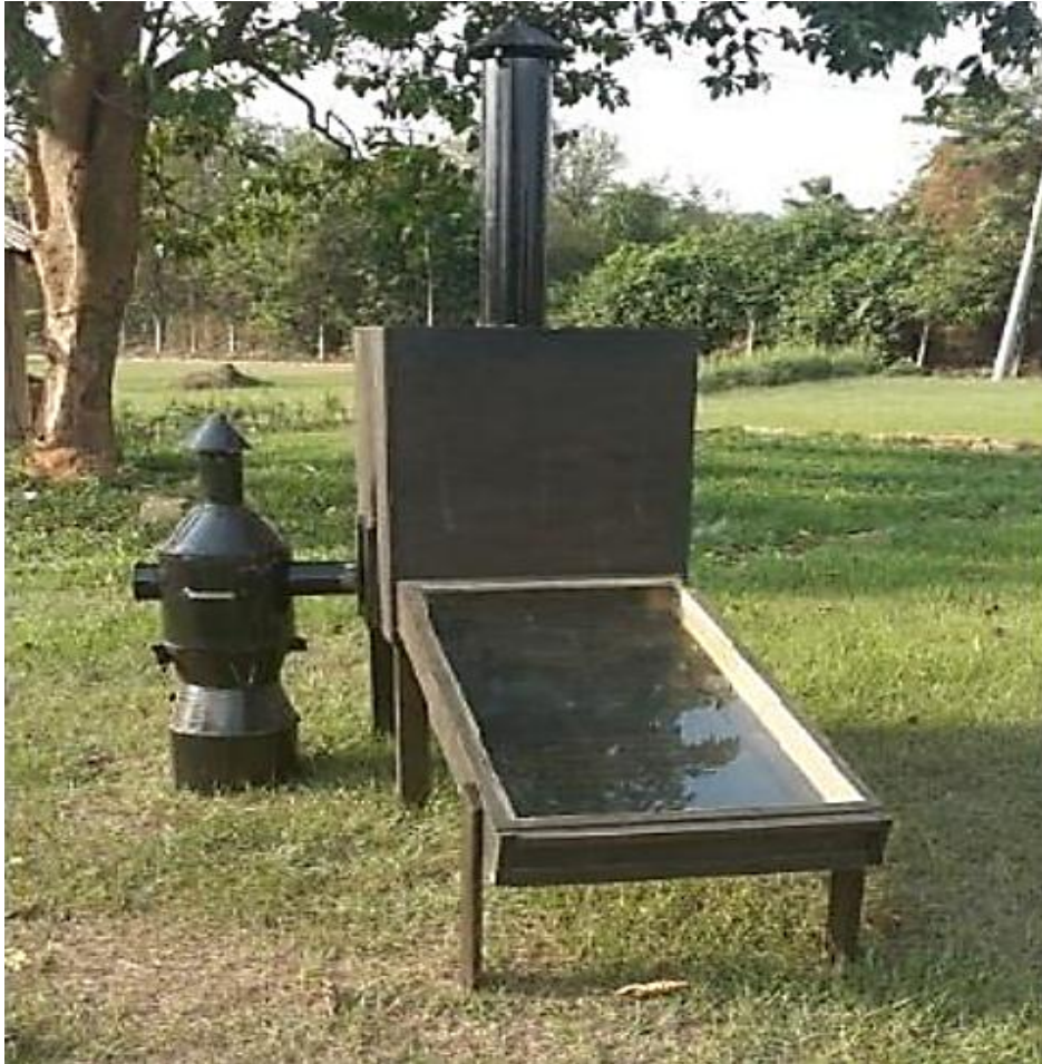
Fig.2.4 Pictorial view of the indirect solar dryer with a backup heater (Tibebu, 2015)
