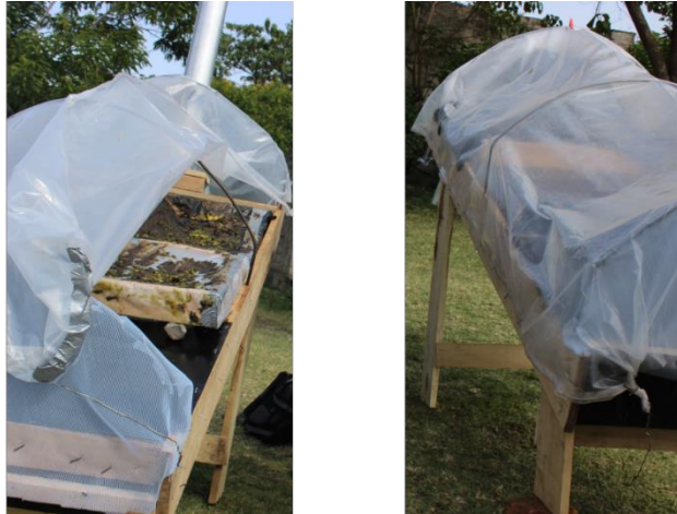
Figure 19. The left image shows how the plastic sheet can be peeled back to assist in tray placement. The right image shows how the dryer can be sealed.
