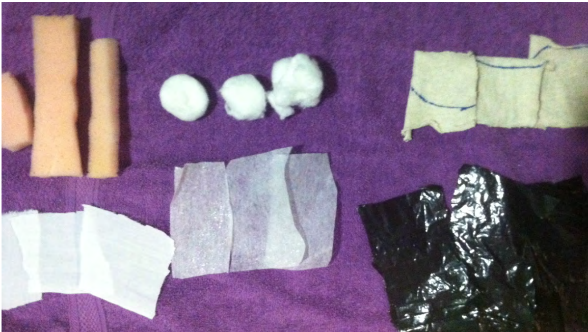
Figure 2: Raw materials used for testing. From left to right by row: foam, cotton balls, mutton cloth, cotton cloth, interfacing/stiffener, and plastic
