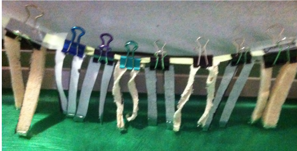
Figure 11: Setup for vertical wicking, four samples for each material. From left to right (two samples per clip): Foam, cotton cloth, mutton cloth, interfacing, mutton cloth, interfacing, foam)
