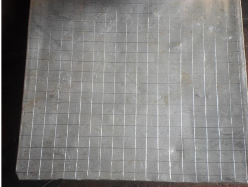
Figure 3.3: Marked out pattern on metal sheet
