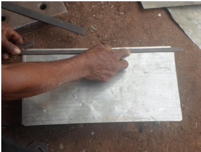
Figure 3.2: Marking out of sheet
