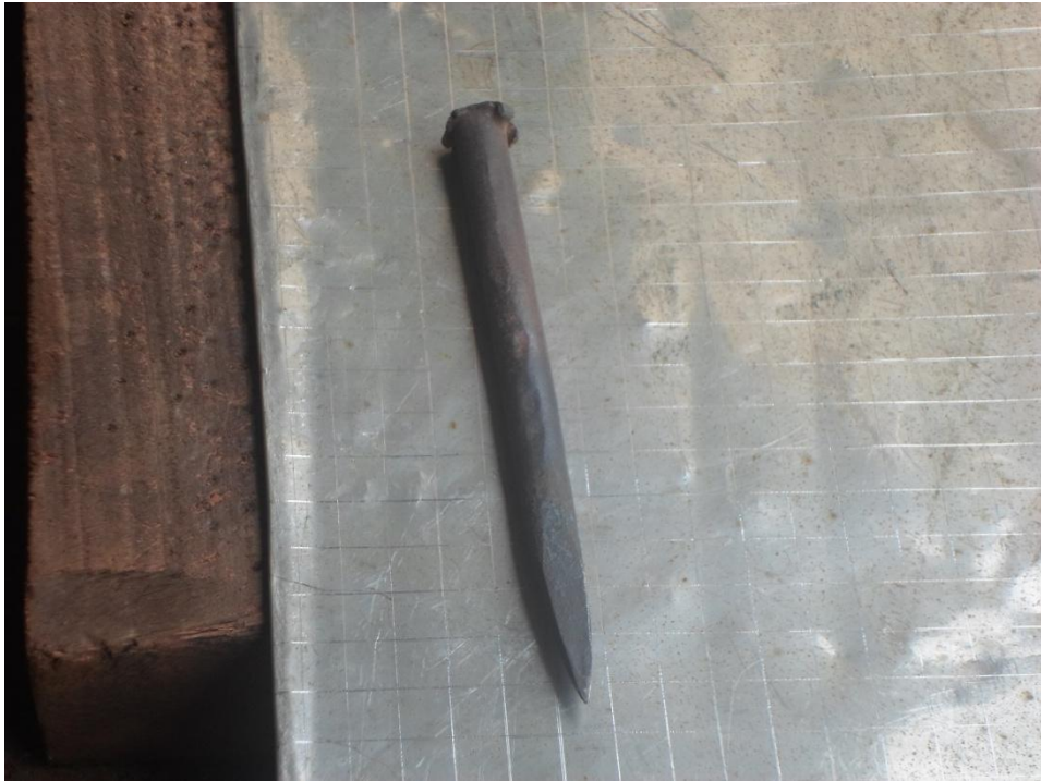
Figure A9: Punch for Making Holes
