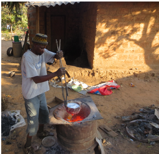
Fig. 1. Casting process in Zambia. Scavenged scrap aluminum is melted down in an iron crucible and stirred with an iron rod. The molten alloy is then poured into sand molds to form pots.
