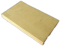
Plywood 20mm thick
