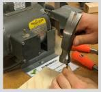
Hold nail at angle, then rotate until perpendicular to the wood.
