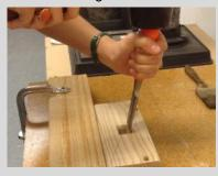
When removing material, chisel toward the center, continuously alternating directions. Redefine the edges as needed.
