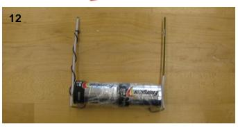
Current travels the path of lowest resistance, not necessarily the desired path. Low resistance materials pull large amounts of current. If too much current goes across the batteries, they will short and get too hot.
