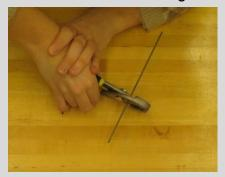
Straighten sharp bends by putting the sharpest point in the pliers' jaw and pulling open the sides.
