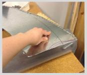
Hit sheet metal against pipe with flat bar. Make incremental changes from right to left to avoid kinks. If kinks appear, change the orientation to flatten them (effectively thinning the metal.
