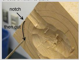
Keep the blade parallel with the saw's frame. Twisting the blade will cause it to break.
