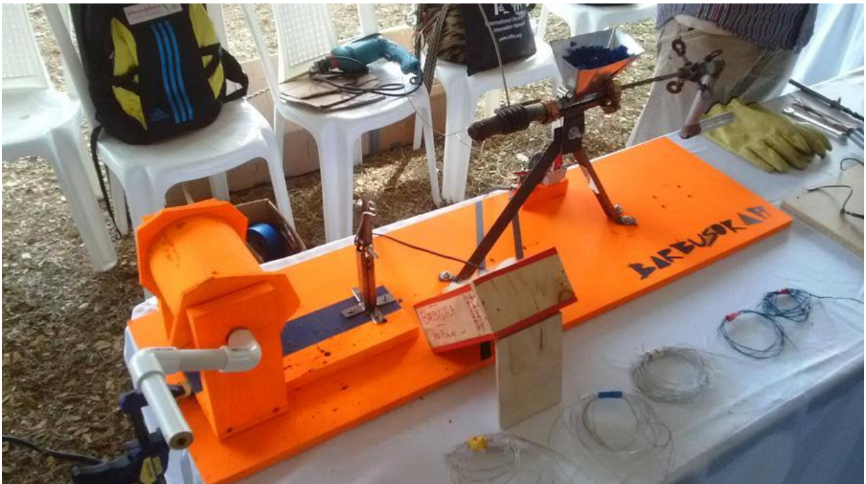
To convert the plastic from pellets to filament a heating element was required. He were are running the first tests on the heating element.
