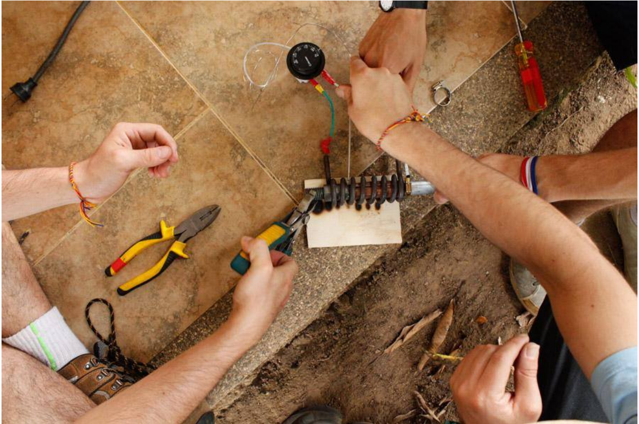
To convert the plastic from pellets to filament a heating element was required. He were are running the first tests on the heating element.
