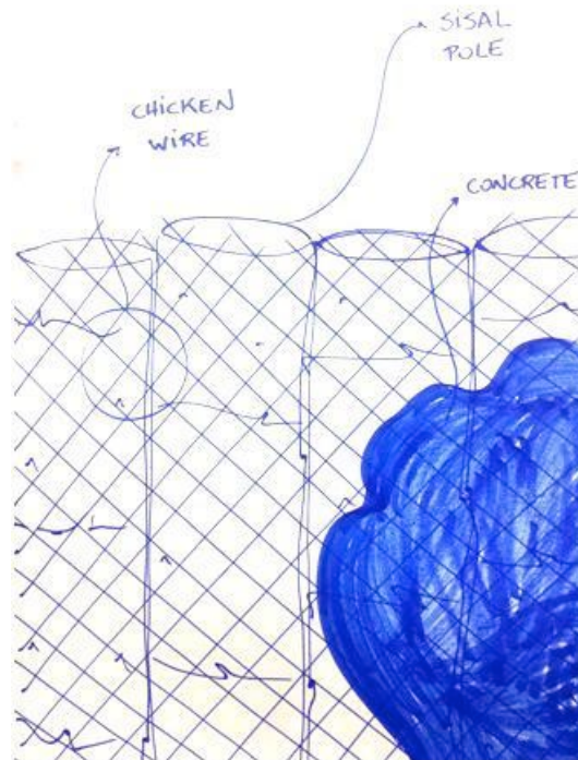
Picture 7: Schematic view of the tank's structure using chicken wire.
