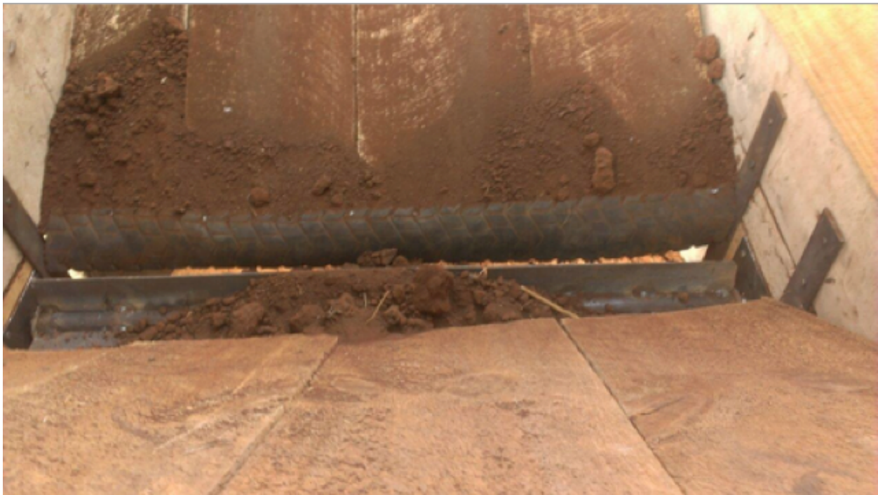
Fig. 4. Top view of the rotating bar and the slopes with some soil after demonstration.
