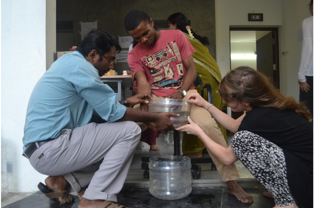
Here, we repurposed a water dispenser tank to demonstrate the way the bell siphon works.
