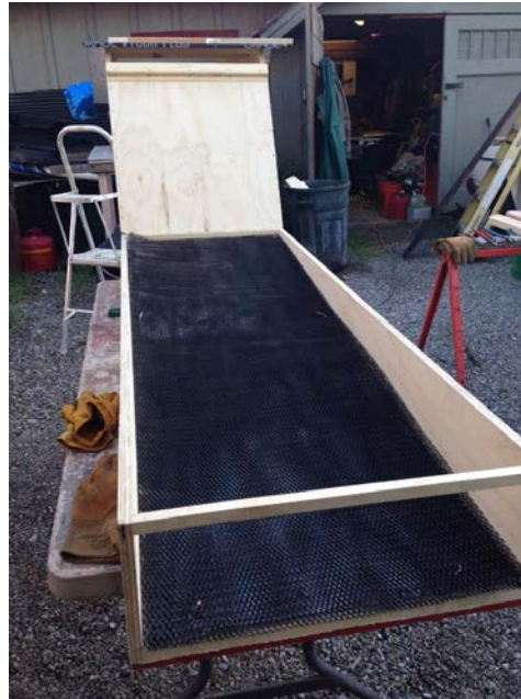
Figure 14: Solar collector box and metal lathe sheet with polycarbonate plastic removed.
