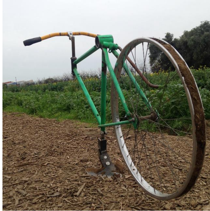
Figure 8: Completed Bike Cultivator (The Green Machine)
