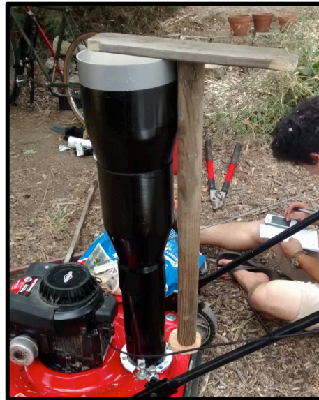
Figure 2. Depicts the main entering hopper and the wooden plunger
