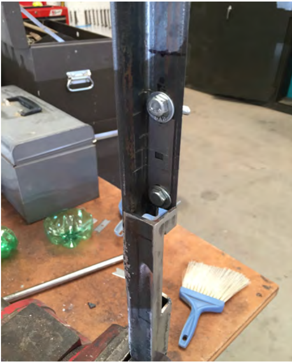
Final design showing inside of angle iron with blade attachment on right side and cutting strip widths on left.
